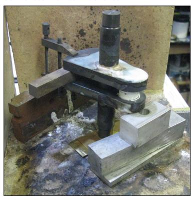
In case you wondered, the white stuff on the crank pin is Tipex. It is a good medium to use to stop solder flowing and it also protects the surface from heavy oxidation when using a lot of heat. I should have put some on the axle bearing areas well but as forgot! Yes I know there are machine marks webs the were cut on
